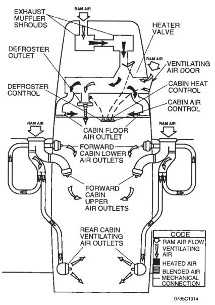
Figure 7-8. Cabin Heating, Ventilating and Defrosting System.
