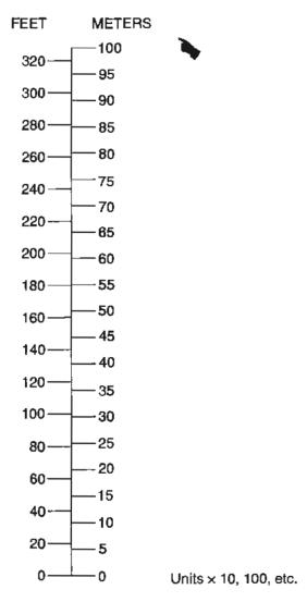
Figure 1-3. Length Conversions (Sheet 2 of 2)
