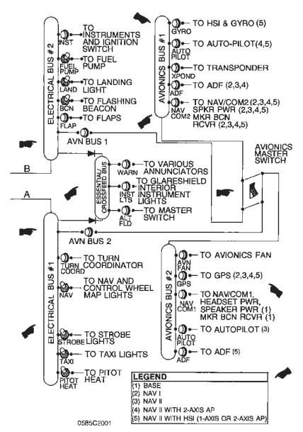
Figure 7-7. Electrical Schematic (Sheet 2 of 2)
