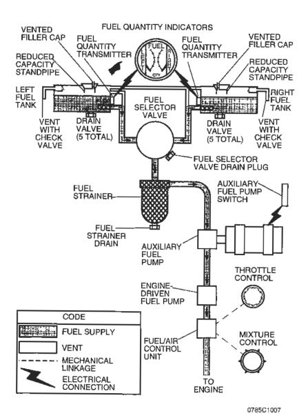
Figure 7-6. Fuel System Schematic
