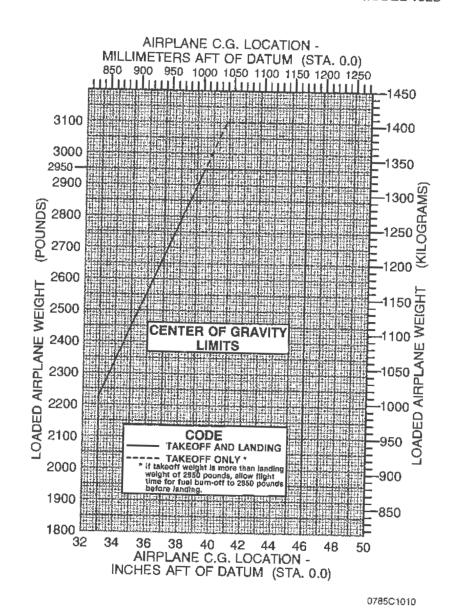
Figure 6-8. Center of Gravity Limits
