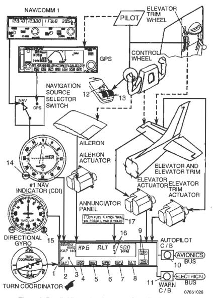
Figure 1. Bendix/King 2-Axis KAP 140 Autopilot Schematic (Sheet 1 of 5)
