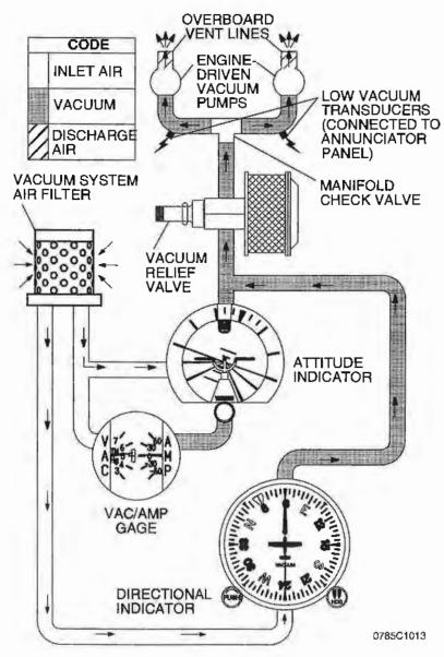
Figure 7-9. Vacuum System Schematic
