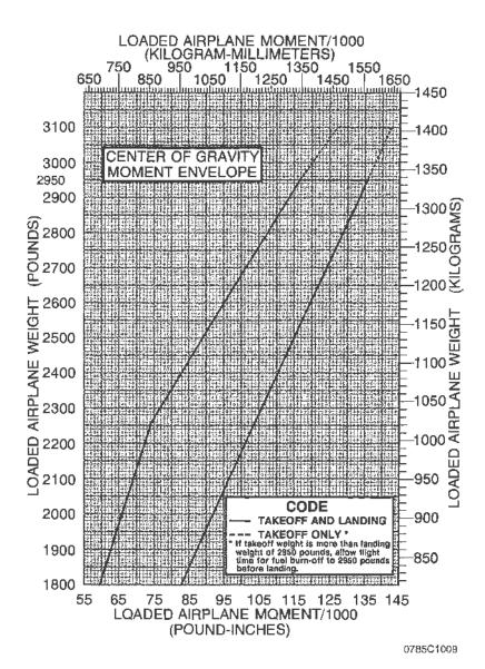
Figure 6-7. Center of Gravity Moment Envelope
